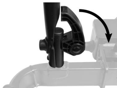
Figure 25: Loosening the quick-release lever
