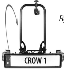
Figure 13: Swinging out the lamp holder
